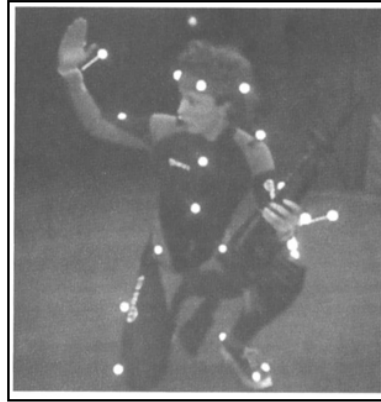
Figure 19: A configuration of 20 motion capture sensors on a human actor, Kerlow (1996, p. 279)
